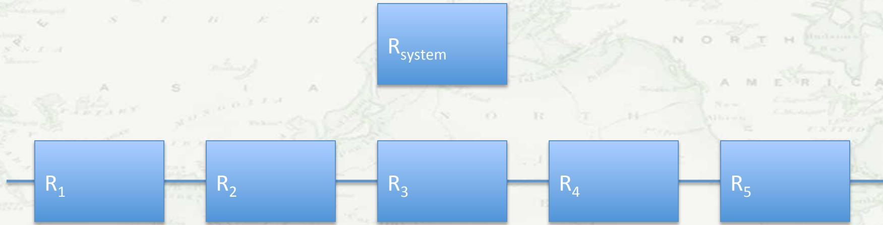
$$R_{\text{system}} = \prod R_i$$
